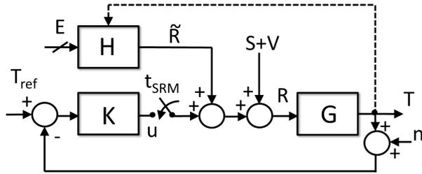
Fig. 1. Block diagram of the solar radiation management (SRM) control problem. Climate model  $G$  with output temperature anomaly  $T$  is driven by net radiative forcing  $R$  comprised of anthropogenic radiative forcing  $\tilde{R}$  from GHG emissions  $E$ , volcanic forcing  $V$ , solar forcing  $S$  and the influence of the SRM controller  $K$  for time  $t \geq t_{\text{SRM}}$ . The dashed line depicts the influence of climate feedbacks on the gas-cycle model  $H$ .
