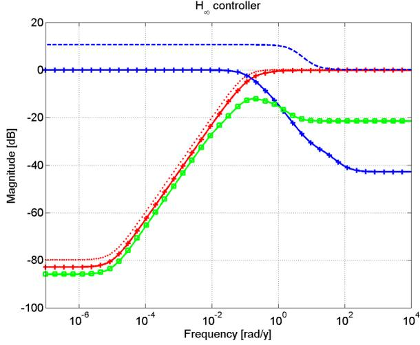
Fig. 3. Sensitivity function (solid, +) with upper bound ( $\cdots$ ), and complementary sensitivity function (solid, o) with upper bound ( $\cdots$ ) arising from the controller  $K_\infty(s)$  in (5). Disturbance-to-output transfer function  $GS$  shown with  $\square$
