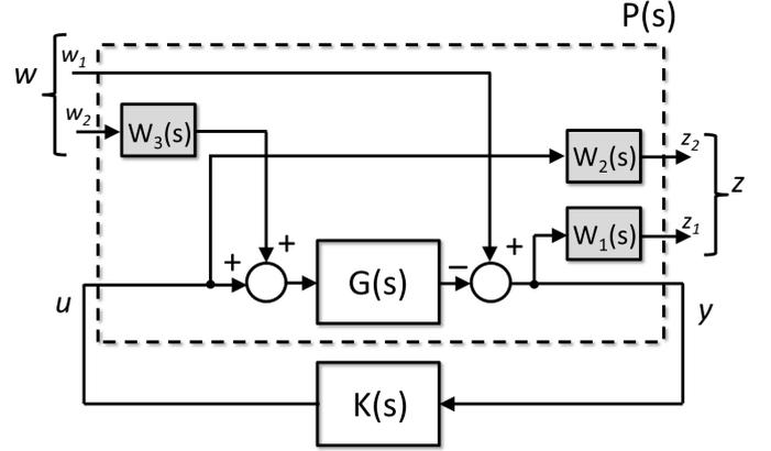
Fig. 2. Augmented system  $P(s)$  and SRM controller  $K(s)$  in standard control configuration. Exogenous signals consist of the temperature reference  $w_1$  and combined anthropogenic/solar/volcanic forcing  $w_2$ , while the error signals are the temperature tracking error  $z_1$  and SRM actuator signal  $z_2$ , weighted by  $W_1(s)$  and  $W_2(s)$ , respectively.
