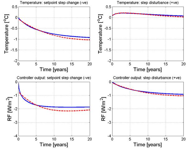
Fig. 4. Time-domain responses for  $H_\infty$  and PI controllers. Response of  $H_\infty$  controller (—); PI controller (---)
