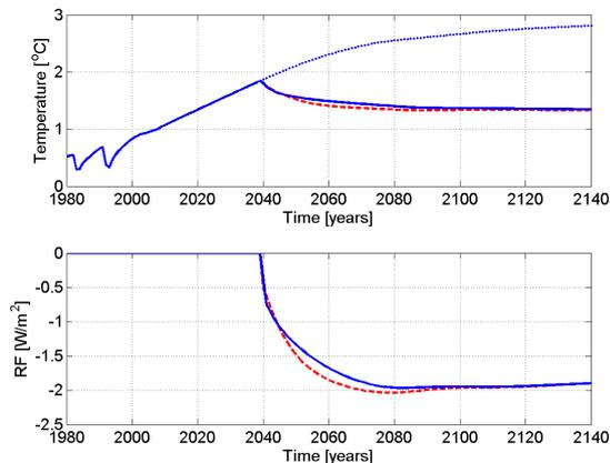
Fig. 5. SRM simulation using MAGICC climate model:  $H_\infty$  (—) and PI (- -) controllers. RCP4.5 temperature projection (· · ·)
