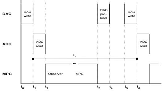
Fig. 4. Controller timing:  $T_s$  is constant and  $t_1$  and  $t_6$  are the sampling “instants”.  $t_0$  (and  $t_5$ ) mark the beginning of a DAC write operation, which preempts a delay so that writing the input and reading the output occur within tolerable margins.
