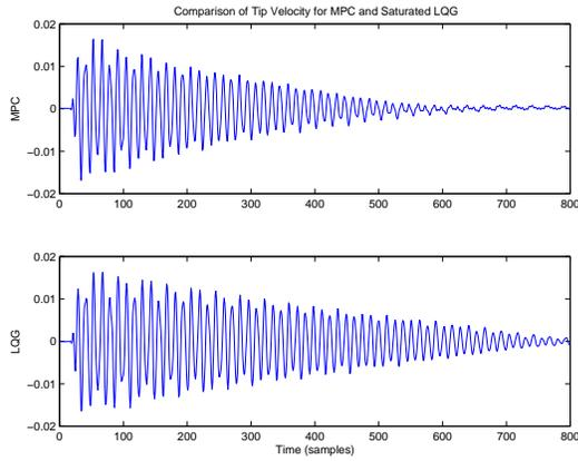
Fig. 6. Comparison of tip velocity for MPC and Saturated LQG (SLQG) running at 5kHz sampling rate when a filtered step function (for 4th mode) is applied to the disturbance patch. Notice a distinct reduction in settling time.
