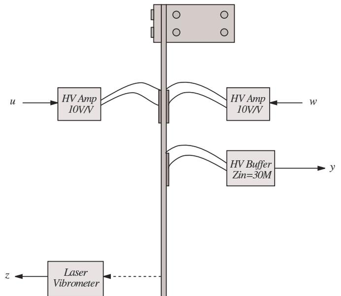
Fig. 2. Plan view schematic of the experimental apparatus.
