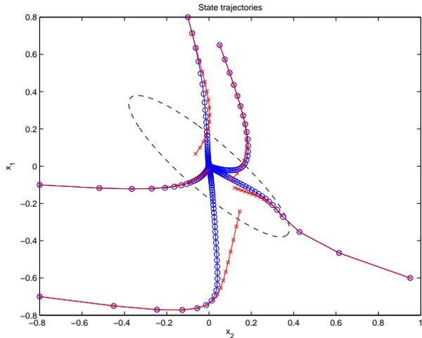
Fig. 2. State trajectories for different initial conditions and barrier weighting  $\mu = 0.1$ ; actual(o), initial prediction(x). The ellipse describes the boundary of  $X_f$ .
