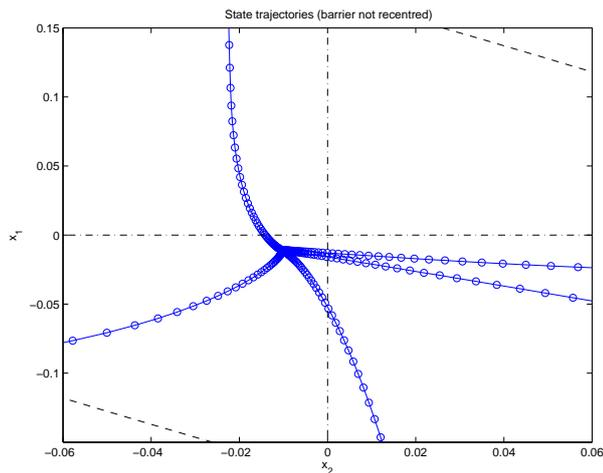
Fig. 5. Close-up of origin with standard logarithmic barrier. Note the trajectories *do not* converge to the origin since the barrier is not recentered in this case.
