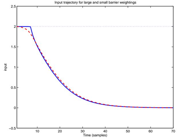
Fig. 3. Input trajectories for different barrier weightings:  $\mu = 10^{-6}$  (solid) and  $\mu = 0.1$  (dashed). Note that the large weighting results in a more cautious control action near constraint boundaries, while the trajectories are similar when away from the boundary.
